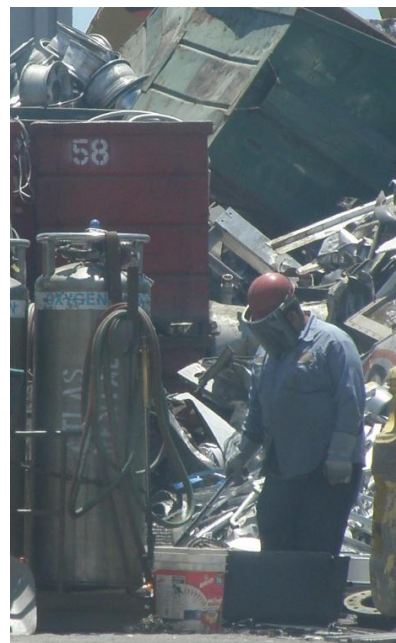
Above: In some businesses, the mechanical preprocessing, such as in this instance of a worker with a welding torch, happens in a scrapyard in the open air.
